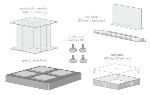
Tightly screw adjustable casters into bottom of quad tower base before assembling.
