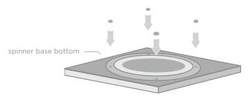
Stack one mag|stak™ module on top of spinner base using alignment disks which set into alignment ports as shown below. Stack second module in same fashion. Ensure a secure and stable fit.
