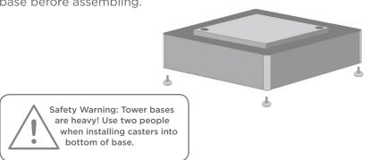
Stack one mag|stak™ module on top of single tower base using alignment disks which set into alignment ports as shown below. Stack additional modules on top, in same fashion.
