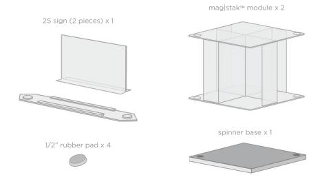
Attach rubber pads on metal plate on the bottom of the spinner base using the smallest holes as placement markers.
