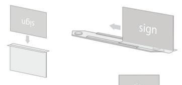
Place signage on top mag|stak™ module, making sure to connect alignment discs with alignment ports. Ensure a secure and stable fit.
