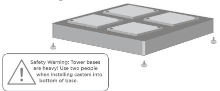
Stack one mag|stak™ module on top of quad tower base using alignment disks which set into alignment ports as shown below. Stack additional modules on top, in same fashion.
