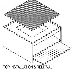
RECESSED SUB-TOP **CUT-OUT FOR ACCESS TO TOP OPENING TO STORE TOYS FIXED SHELF** STORAGE COMPARTMENT FOR SECOND TOP NOTCH IN BOTTOM PANEL FOR HAND-HOLD TO REMOVE "STORED" TOP LOCKING CASTERS
