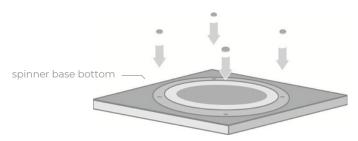
Stack one magstak™ module on top of the spinner base using the alignment disks that set into alignment ports as shown below.
