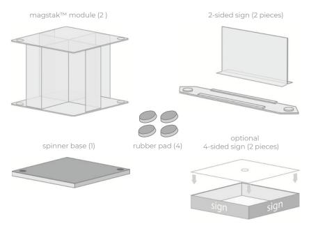
Attach rubber pads on metal plate on the bottom of the spinner base using the smallest holes as placement markers.
