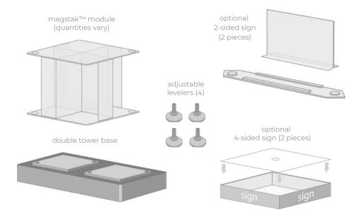
Tightly screw adjustable levelers into bottom of double tower base before assembling.
