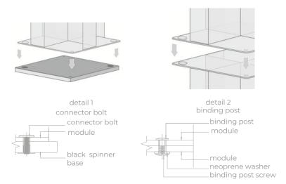
Optional: connect bottom module to spinner base using connector bolts (see detail 1). Stack second module in same fashion and connect the two modules using the binding post, neoprene washer and binding screw (see detail 2) to ensure a secure and stable fit. Do not over tighten!
