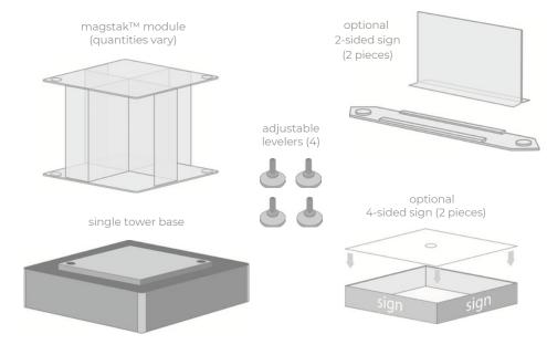
Tightly screw (4) adjustable levelers into bottom of single tower base before assembling.
