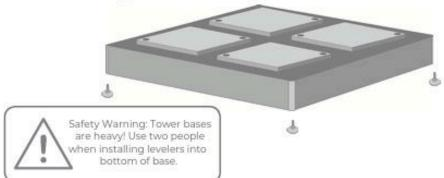
Stack one magstak™ module on top of the spinner base using the alignment disks that set into alignment ports as shown below.
