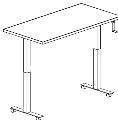
Hand-crank, adjustable height (29" - 42" AFF) / caster base
