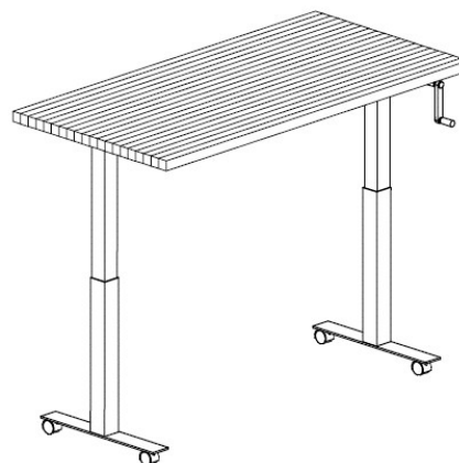
Hand-crank, adjustable height (30" - 42" AFF) / caster base
